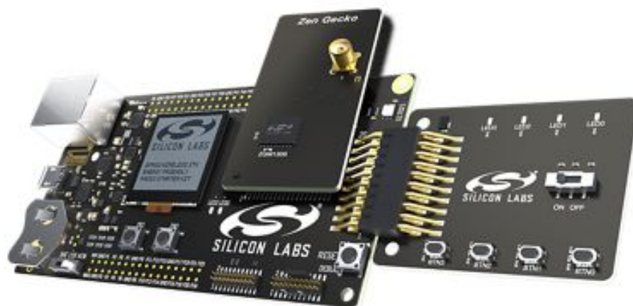
Figure 1: Main Development Board with Z-Wave SiP Module
