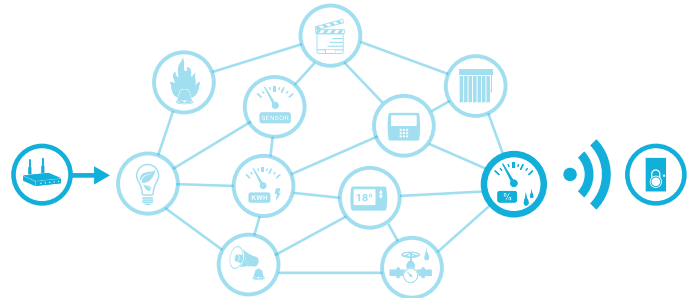
Figure 2. Last repeater in path sends wake up signal to door lock
